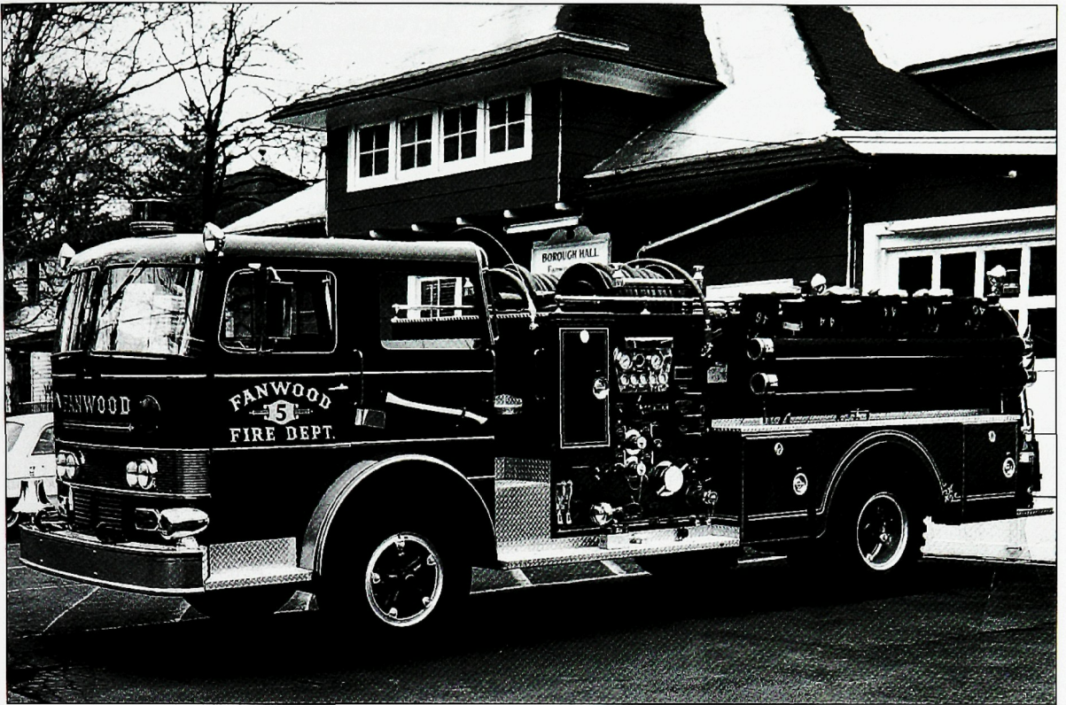
UP TO DATE. Fanwood's first modern truck, Engine No. 5, was a triple-combination cab-over-engine designed by Great Eastern.
