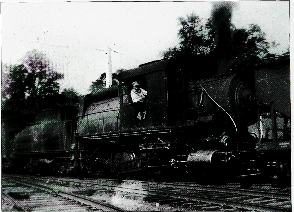
RAILROAD VIEWS. A small engine, known as a shunting engine, moved railroad cars to and from the sidings onto the mainline tracks.
