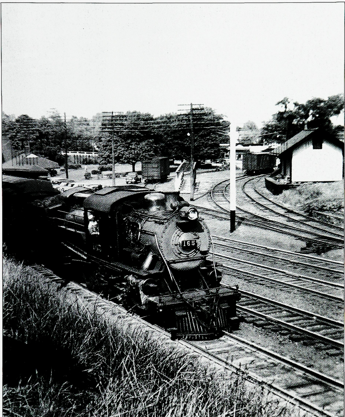
THE RAILWAY SETTING. A camelback engine at the head of a passenger train pauses in the westbound lane at the Fanwood station. Three railroad sidings can be seen in this 1940s photograph. The siding at the far right served the white freight station. The left two sidings, each hosting a freight car, ran across South Avenue to bring bulk materials into the coal and lumber yards.
